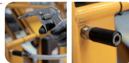
| Air line in platform
