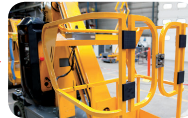
| Swing gate entry
