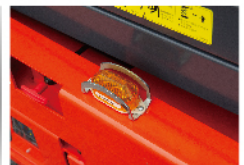
Emergency falling and dual flashing warning lights
