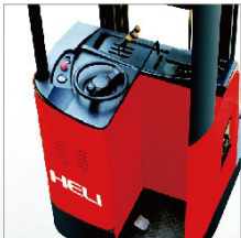
Large cab with dead man power off switch, Multi-function display: battery state, hour metre, fault indicator etc.
