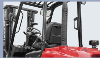
**4.** The new design mast provides broad forward visibility due to the longer distance between inside mast.
