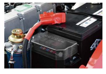
Adoption of new generation integrated electric box makes maintenance and repair convenient, layout becomes more reasonable and with better water-proof performance.
