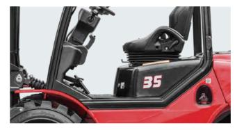
The easy-to-open hook provides quick access to the engine compartment.
