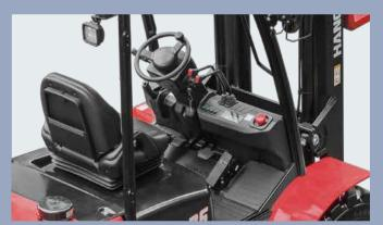
2. The extra foot space is provided to reduce operator fatigue significantly, non-slip step makes getting in and out easy an safe. The new designed steering wheel new brake system and the easy-to-operate levers provide total handling operation.
