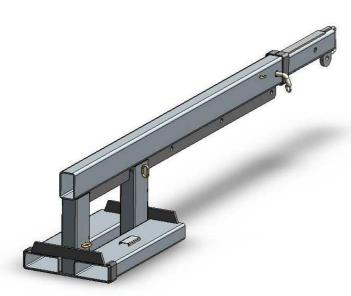
The type FJL2.5 Fixed Jib (Long) is designed as an affordable general purpose Jib with a 3.5 metre reach when fully extended. This slip-on Forklift attachment is held to the Forklift by a safety chain. The Jibs overall length when closed is 2.1 metres.
