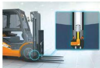
■ lowering buffering device
